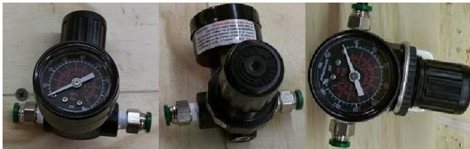
Figure 8 - Main regulator plumbing
