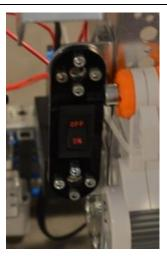
Power the robot "Off" using the Main Power Switch. The team's Main Power Switch should be clearly labeled, as outlined in the Robot Inspection Rules. Make sure the robot remains off for a minimum of 5 seconds.
