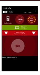
Have the team verify that the driver station is connected to the control hub and that there are active ping times being displayed on the main driver station screen.
